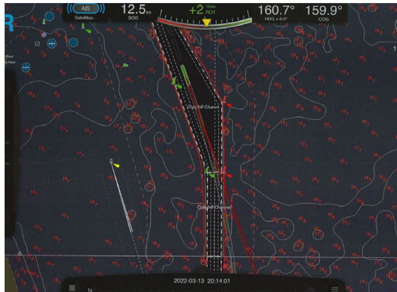
Figure 5. PPU screenshot just before the end of the first recording of EVER FORWARD's transit at 2014 on March 13, 2022, just prior to the grounding. Image provided by Pilot 1.
