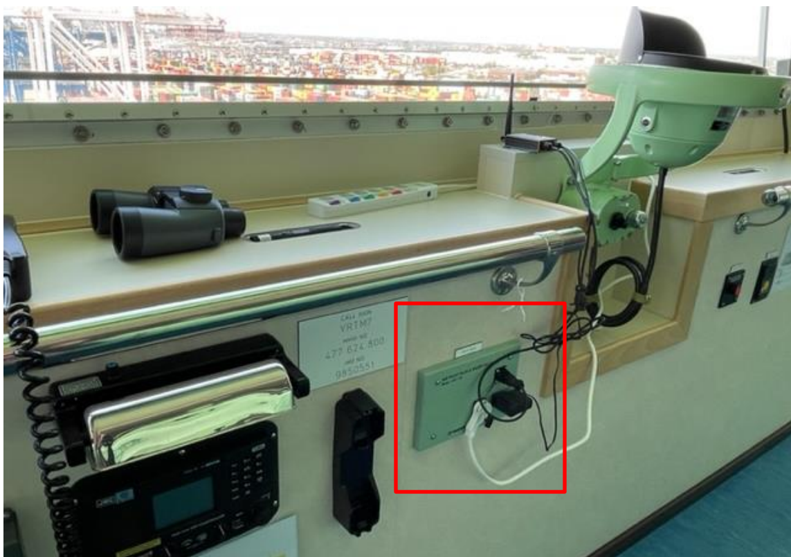
Figure 2. The red square shows the location of EVER FORWARD’s Pilot Plug. This photograph was provided by Association of Maryland Pilots and taken in Baltimore, Maryland.
